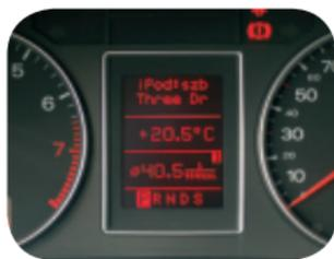
The menu of the Gateway Pro is displayed on the central display (cluster) on the dashboard (between the two main instruments). Due to the capabilities of your car, the Gateway Pro menu or song info (id3) is not visible on the radio screen.
